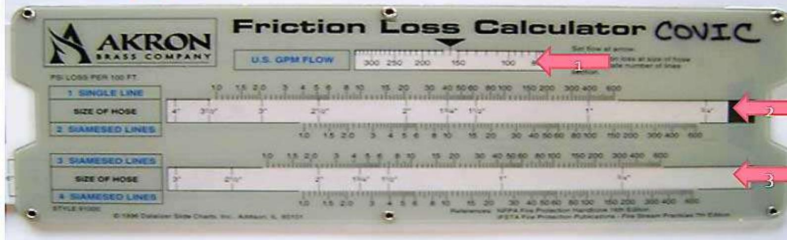
The list of black numbers just below line 2 would be the numbers you would use if you were using multiple lines to supply the given flow rate. For example, if you were using 2 lines to flow our 160 gpm, (we were using 1 3/4" lines) the friction loss would be 10 psi. You do have to use the same size lines to use this part of the slide calculator. Line 3 would be used for 3 or 4 lines to supply a given flow rate.
